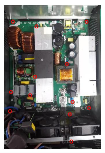
**Note:** When you put the new control board on the main board, please make sure that the connection is correct and tighten. Don't forget to put the screws and cables back.
