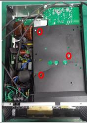
Remove the nine screws, then Remove the MPPT board on the side;
