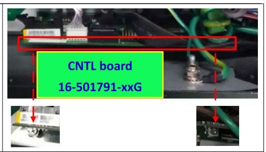
Remove all cables here(AC In/Out cables, GND cables, Signal cables FAN cables). Brown cable is line;
