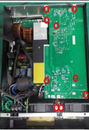
Remove the cable from the control board;
